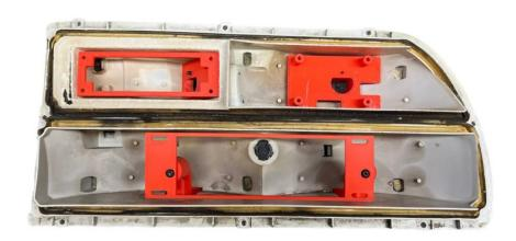
Attach the end caps on the backside of the housing and securely fasten with the included M3x8 screws.
